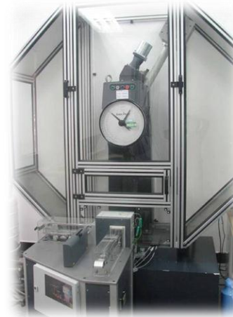
Material impact test machine
