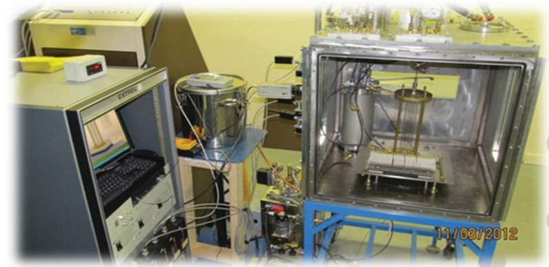
LOCA high temperature oxidation and quench simulation test facility
